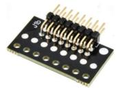
Solder the 2x8 pins, 90° connector J1b on PCB-5.
