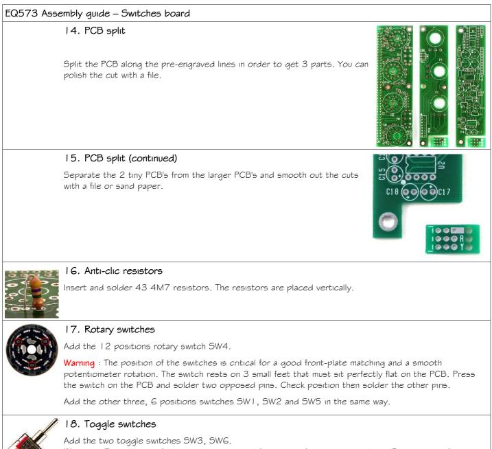
**Warning** : The position of the switches is critical for a good front-plate matching. They must sit flat on the PCB. Press firmly the switch on the PCB and solder two opposite pins (housing). Check position then solder the other pins.
