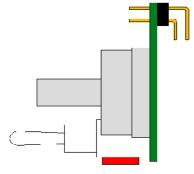
Now solder all the pins on the external row. Cut the soldered pins flush, in order to get access to the second row. Solder the second row then cut the pins flush.
