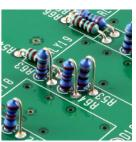
**Warning** :Some resistors are placed vertically. Bend one leg 180° and insert. The horizontal resistors must be bended at 0.4".
