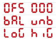
Blinking between OFS and value : Adds an offset between -12 and +12 dB to the input signal.
