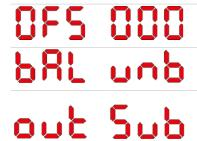
Blinking between OFS and value : Adds an offset between -12 and +12 dB to the output signal.
