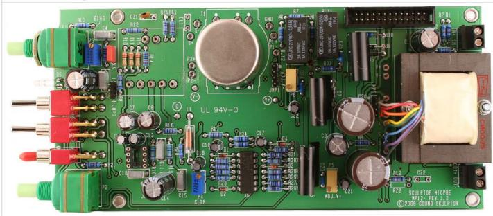
After your board has been stuffed, brush the solder side with a hard tooth brush to remove any remaining solder bits. Make a full visual check. Any missing component on the board? Any remaining component in the box? When everything is correct, install the input and output XLR's as described in the SKMP Assembly Guide. Your MP12 is now ready for test and setup. Please follow instructions in the "MP12 Setup" document.
