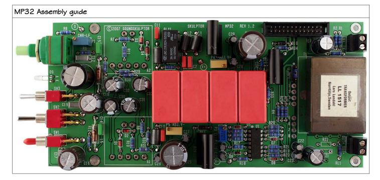
After your board has been stuffed, brush the solder side with a hard tooth brush to remove any remaining solder bits. Make a full visual check. Any missing component on the board ? Any remaining component in the box ? When everything is correct, install the input and output XLR's as described in the SKMP Assembly Guide. Your MP32 is now ready for test and setup. Please follow instructions in the "MP32 Setup" document.
