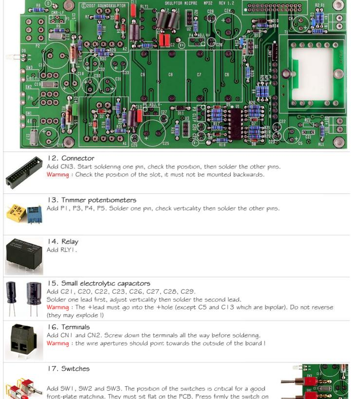
Add SW1, SW2 and SW3. The position of the switches is critical for a good front-plate matching. They must sit flat on the PCB. Press firmly the switch on the PCB and solder one of the front pins (housing). Check verticality and horizontality. Then solder the other pins.
