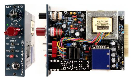
A Direct Instrument, high impedance, input is available on the front. A relay is automatically switched when a jack is inserted. It connects the DI signal to the input transformer of the preamp.
