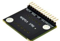
Use the input transformer front PCB, the one with the pin holes and numbers. Insert the 90°, 13 pins headers, long tails first, into the holes, from the bottom side, marked "Not visible".
