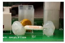
For security, hide the exposed wires of the thermal fuse with some silicon sealant.
